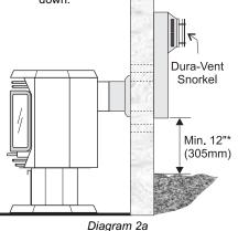
\*Dia 2a & 2b: As specified in CGA B149 Installation Code. Local codes or regulations may require different clearances.
